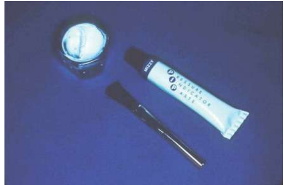
Figure 5.1.6. Commercially available pressure indicator paste dispensed in a dampen dish to be applied with a disposable bristled brush.
