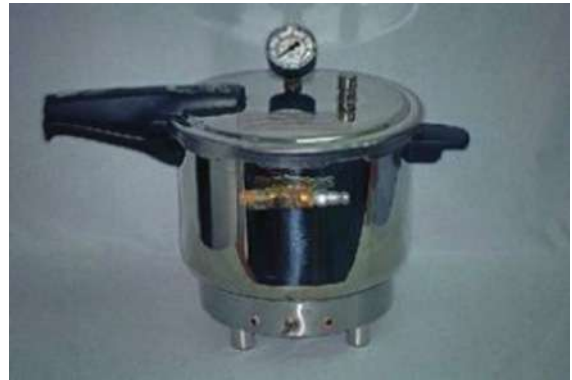
Figure 5.2.14. A pressure cooker or pressure pot is an effective method of curing autopolymerizing acrylic resin. A denser and stronger cure is possible compared to "air curing." However, heat-activated polymerized acrylic resin has greater density and strength than auto-cured polymerized acrylic resin.
