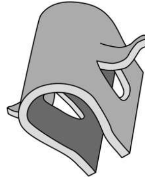
Figure 6.2.24. Metal clip (matrix) snaps onto a bar.
