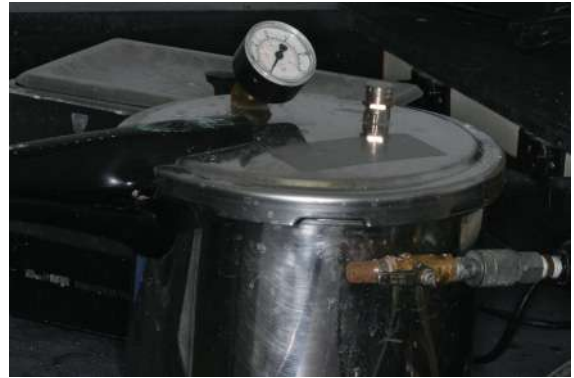
Figure 6.1.18. A pressure pot can be used with a chemical-cure resin to reduce the incidence of porosity in the interim prosthesis made of resin only.
